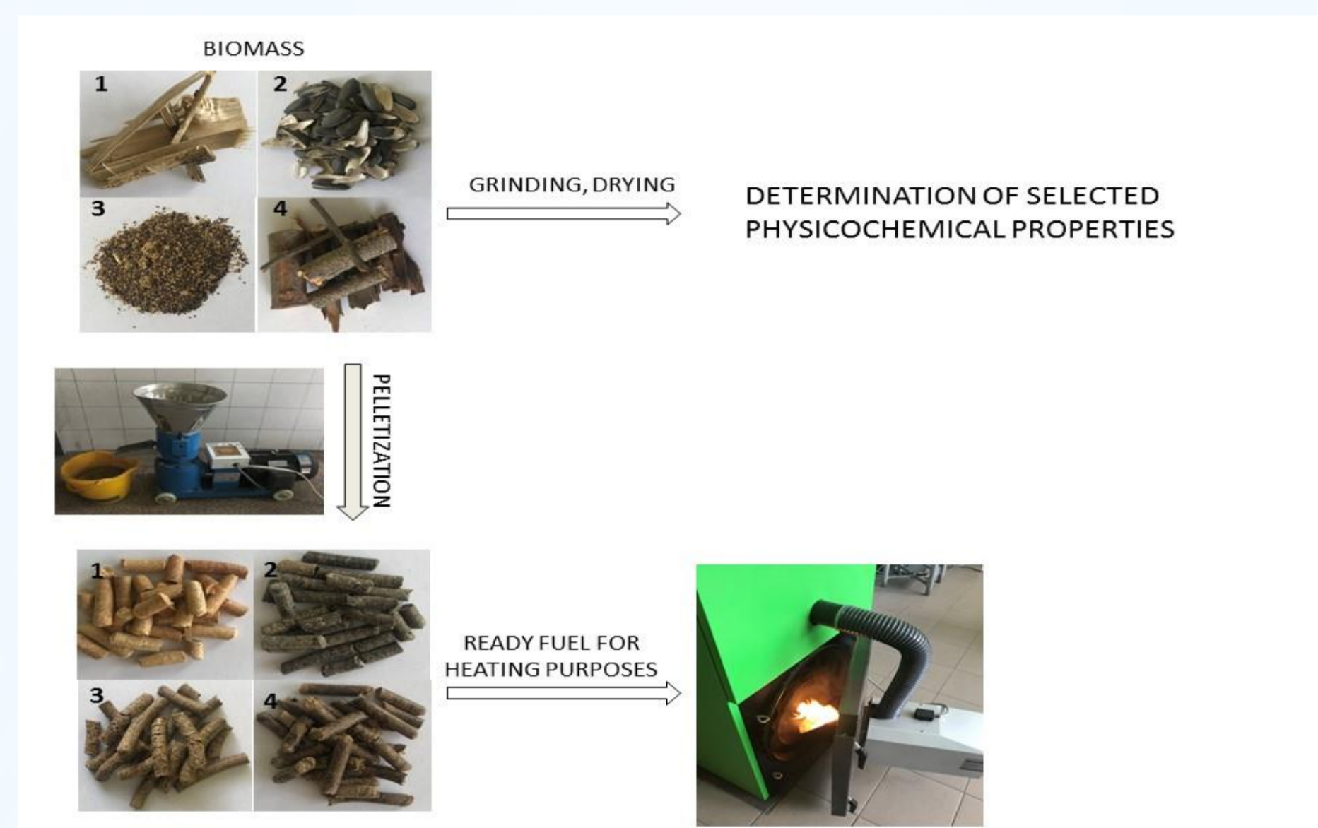
FIGURE 1. Schematic diagram of use of selected types of biomass as a heating fuel, where: 1 - pine, 2 - sunflower husk, 3 - rapeseed cake, 4 - willow ( Salix viminalis )
